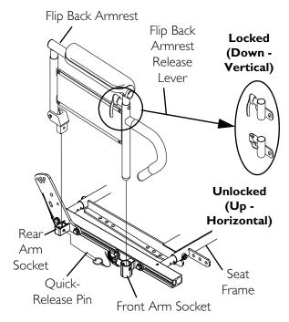
FIGURE 7.1 Installing/Removing Flip Back Armrests
